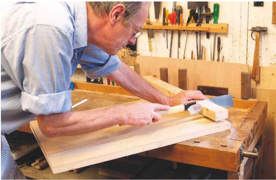
Pic.14 Cut the fence leaving the pencil line in the waste
